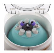
Step 4 — Place the two blood tube adapters in the empty slots, place your blood tube in one of these adapters and a balance tube in the other (See Picture Left). The blood tubes will protrude from the adapter by approx. 2.5cm.
