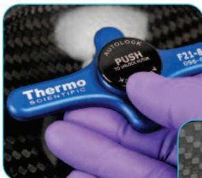
Auto-Lock is identified on Thermo Scientific superspeed centrifuges with a **black push button** and on Thermo Scientific general purpose centrifuges with a **green push button**.
