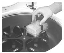
Make sure the rotor is uniformly loaded!
