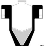
The adapters 70060302 supplied with the cell culture buckets are for use with flatbottomed conical tubes.
