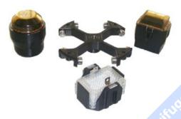
The various swinging buckets are split up into weight categories. These can be identified from the letters suffixing the order number on the bucket. Buckets of identical weight categories should always be installed in opposing positions to avoid imbalance.
