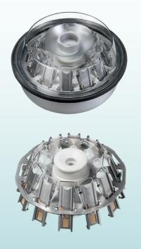
**Special rotors for cytology:** 12 cytological preparations in a single step – rotor 1515 with lid (above) and disk rotor 1520 enable this.
