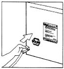
Check main lines and frequency: They must correspond to the values shown on the instrument identification label.
