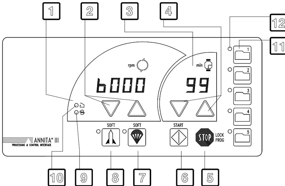
1. **Speed display (units of rpm)** When the machine is stopped, this field displays the set speed. When the machine is running and the numbers are constant, this field displays actual speed. When the machine is running and the numbers are flashing, this field displays set speed.
