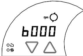
SET **speed** 300 to 6000 rpm (see 4.2 for rotor speed ratings).
