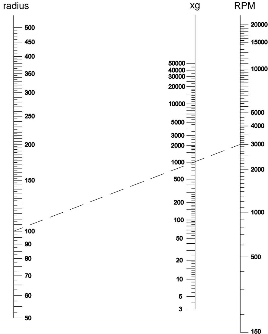
Total separating force applied to a sample in a centrifuge depends on the duration of the centrifuge run and on the RCF (relative centrifuge force) applied to the sample. RCF is generally calculated in units x gravity (x g). The diagram above allows you to graphically calculate RCF by drawing a line from the centrifugal radius (on left) to the speed (on right). The value of the RCF (xg) applied to the sample is approximated by the value at the point where the line crosses the “xg” axis (center).
