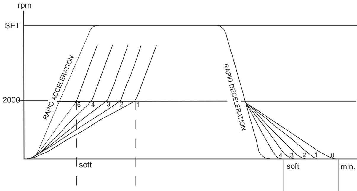
figure 5.4 Acceleration & Braking
