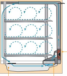
Incoming air first travels over a direct heated water reservoir resulting in 50% faster humidity recovery than
