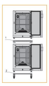
Units are easily stackable. Required stacking adapter provides efficient heat dissipation to operate Steri-Run in one unit while culturing in the other without process disruption.
