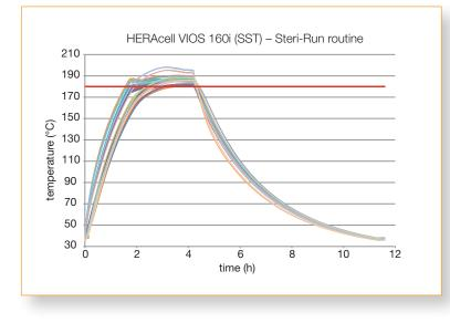
The U.S. and E.U. Pharmacopeias no longer recommend a given temperature and time for sterilization. Instead, they require proof of performance. To meet requirements of a 12 log SAL, a 6 log reduction of biological indicator endospores must be demostrated in half the time.
