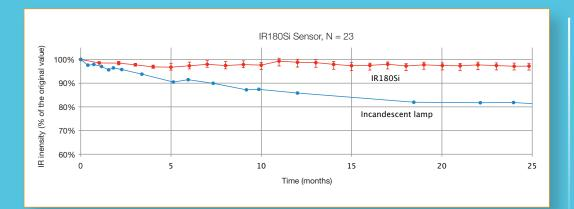
A traditional IR sensor contains an incandescent bulb that puts out less light as it ages, resulting in sensor drift. The IR180Si eliminates this problem. Our silicon MEMS emitter is designed to retain intensity over time, lasting up to 50% longer than ordinary IR sensors.
