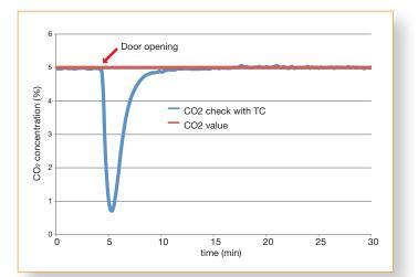
$TC180 - CO_2$  recovery under 6 minutes from a door opening of 30 seconds.
