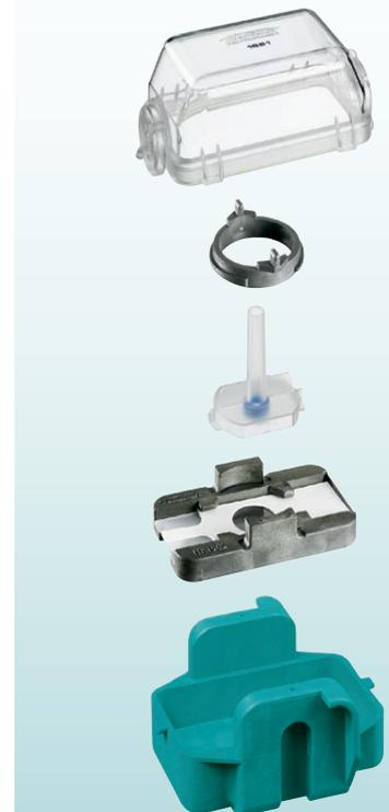
**Assembly of a complete cyto insert with carrier 1660 for cyto chambers.**
