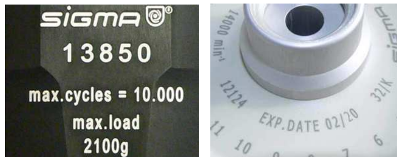
Fig. 4: Different service life – engraving on the bucket/rotor
