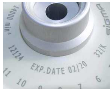
Fig. 6: Different service life – engraving on the bucket/rotor
