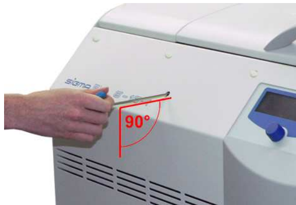
Fig. 32: The emergency lid release key must be inserted horizontally (similar to illustration)
