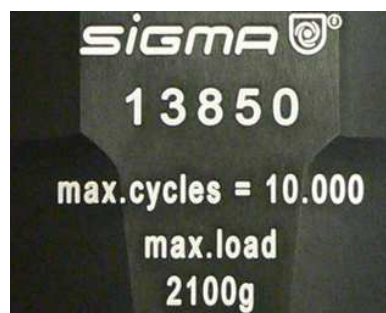
Fig. 6: Different service life – engraving on the bucket/rotor
