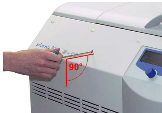
Fig. 31: The emergency lid release key must be inserted horizontally (similar to illustration)
