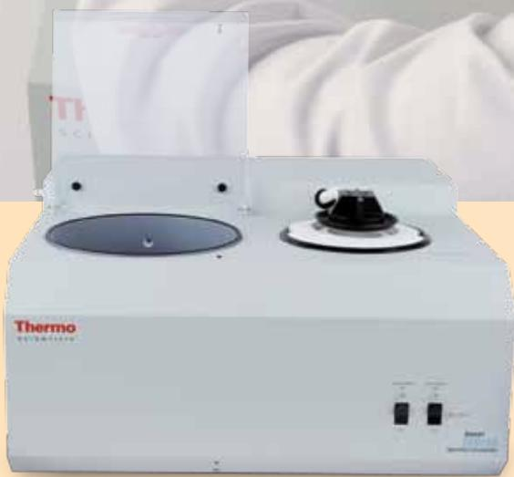
ISS110 P1 SpeedVac Kit includes built-in cold trap, pump, 64 x 1.5 mL rotor and 1L bottle of Thermo Scientific CryoCool heat transfer fluid
