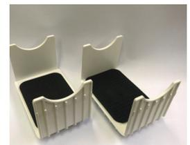
Image 8 - Microplate Adapter
