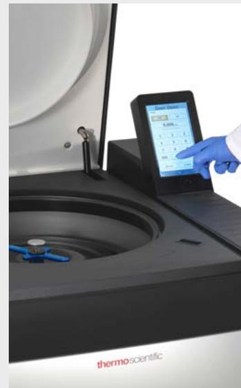
1. Place rotor into the centrifuge chamber
