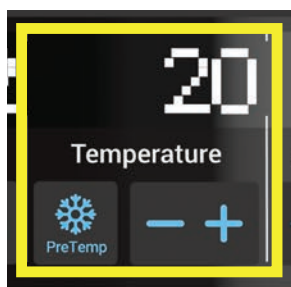
Figure 4-6: Setting the Pre-cooling or Pre-warming Temperature (left)
