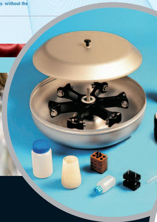
Our Heraeus Cryofuge centrifuges work with the Thermogenesis® AXP™ system to automatically separate cord blood into a freezing bag (for the mononuclear cell product), an erythrocyte bag and an excess plasma bag.
