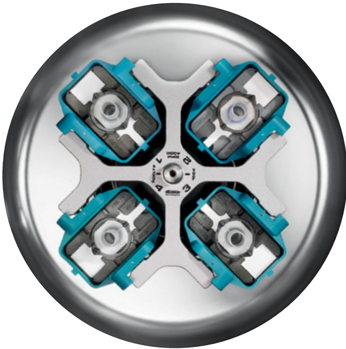
View into the centrifuging chamber showing the rotor 1624 with carriers 1660 for cyto chambers
