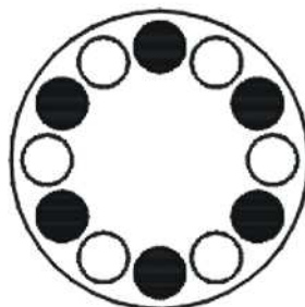
Fig. 7: Permissible and impermissible loading of an angle rotor (example illustration)
