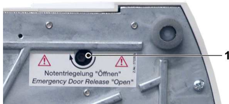
Fig. :10 Opening for the emergency lid release at the bottom of the centrifuge
