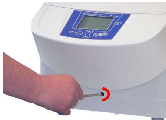
Fig. 11: Manual release of the lid lock
