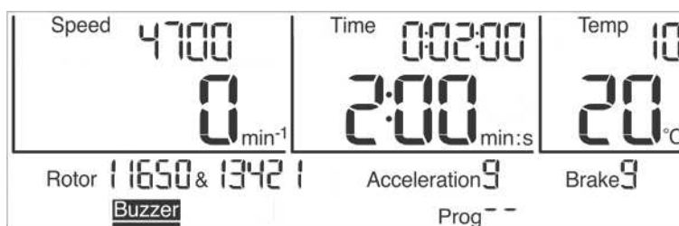
Fig. 20: The sound signal "Buzzer" is activated
