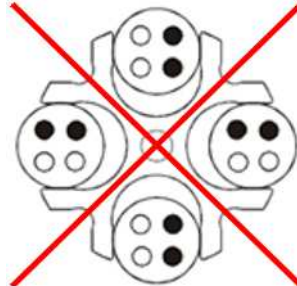
Fig. 7: Permissible and impermissible loading of an angle rotor and a swing-out rotor (example illustrations)
