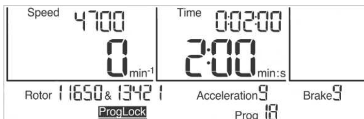
Fig. 20: The program lock "ProgLock" is activated
