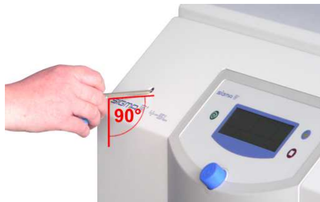
Fig. 27: The emergency lid release key must be inserted horizontally
