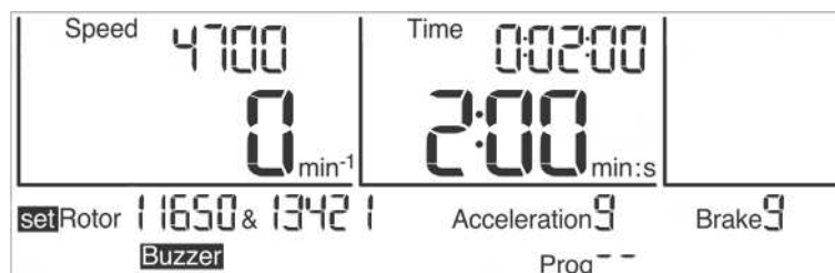
Fig. 16: Preselection of a rotor or a rotor/bucket combination
