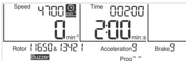
Fig. 13: The function "Runtime as of the set speed" is activated
