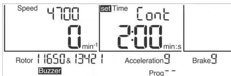
Fig. 14: Indication "Cont" during a continuous run
