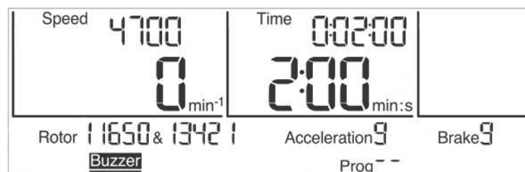
Fig. 19: The sound signal "Buzzer" is activated
