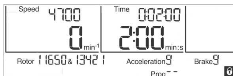
Fig. 23: "Padlock" symbol indicating an activated input lock
