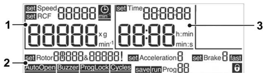
Fig. 10: Display of the "Spincontrol L" control system
