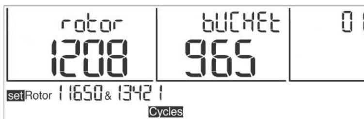
Fig. 21: Cycle display for rotor 11650 and bucket 13421
