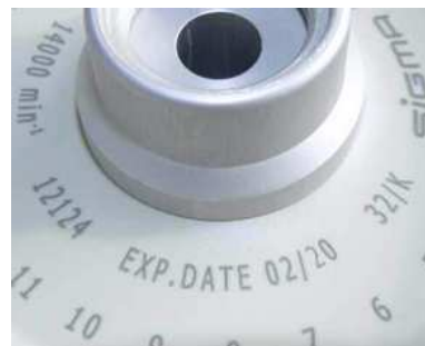
Fig. 4: Different service life – engraving on the bucket/rotor
