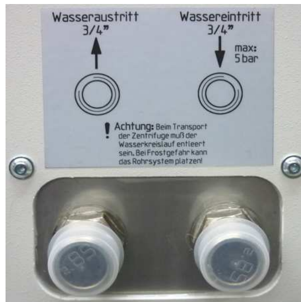
Fig. 7: Connections for the cooling water system
