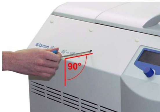
Fig. 33: The emergency lid release key must be inserted horizontally (similar to illustration)
