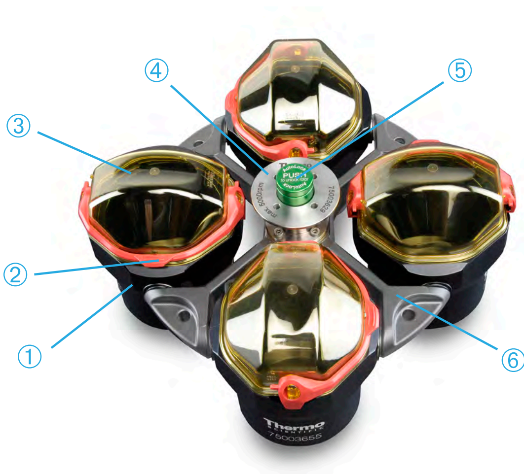
① Bucket; ② Cap latch; ③ Bucket cap; ④ Rotor knob; ⑤ Auto-Lock button; ⑥ Rotor cross
